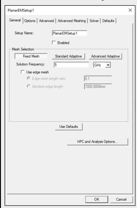
When an analysis setup is deactivated, any sweep associated with it has no effect, even if an associated sweep is enabled.
